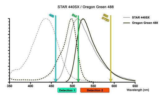
For the spectral separation of two dyes with similar emissions different excitations are required. This is realized by using large Stoke's shift dyes (BD V500 and STAR 440SX) with absorption spectra located in the violet/blue range.
