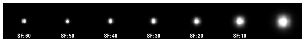
Fig. 2 Compilation of a series of calculated PSFs (Operations Window → Theoretical PSF) with different saturation factors (SF) showing an increasing (but not linear!) full-width-half-maximum (FWHM) value. Pixel size: 15 nm
