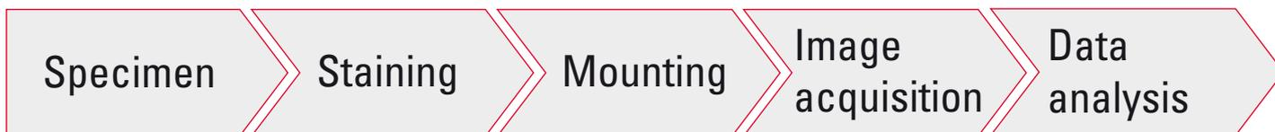
The following sections describe the steps to acquire a high quality STED image. These steps are not significantly different from conventional confocal microscope practice. This starts with the appropriate labeling of the structure of interest by a STED-suitable fluorescent dye. Subsequently, the sample needs to be **embedded**
