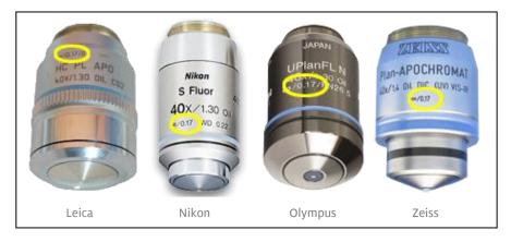
of glass is factored into the optical calculations when the lens is designed. Plastic coverslips and/or culture dish bottoms are <u>not</u> acceptable substitutes for a glass coverslip.
