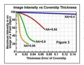
Commercially available coverslips come in a variety of thicknesses, but the thickness closest to 0.17mm is a #1.5 coverslip. For the newer, superresolution optical microscopes, a #1.5H (high performance) is the required thickness. Using the incorrect coverslip thickness can greatly reduce your ability to get the most information out of your sample using an optical microscope.
